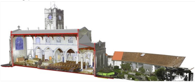
Example of 3D model developed from point clouds
